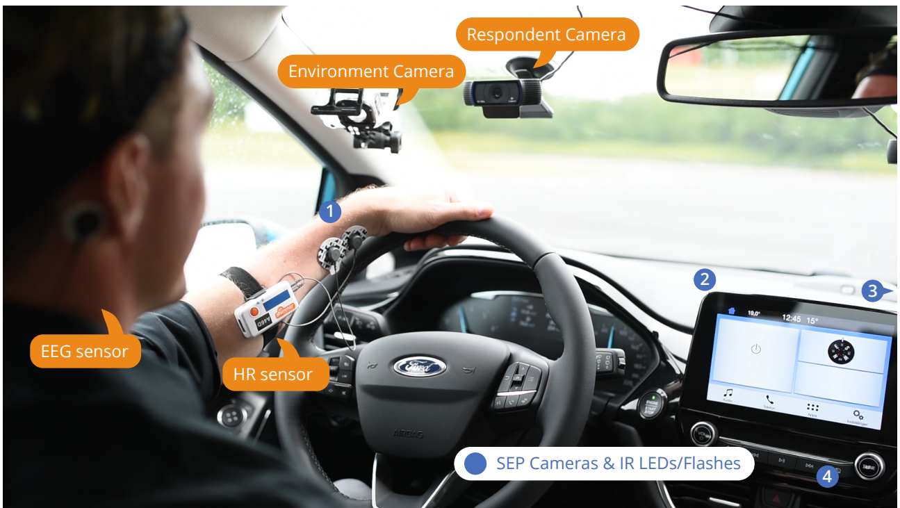
Example of setup with iMotions and Smart Eye Pro
